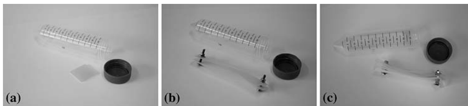
Fig. 2 Setup of the samples in each assay. (a) Squared plate; (b) films of 0.5 mm and (c) films of 0.15 mm
